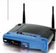
ACCESS POINT (Wi-Fi connection)
