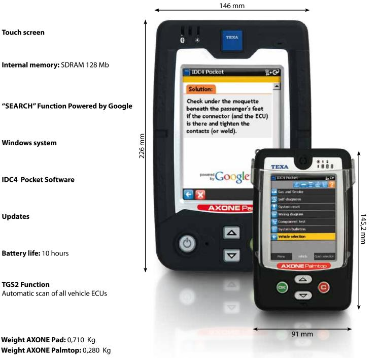
Screen AXONE Pad: TFT 5,7', 65.536 colour QVGA Screen AXONE Palmtop: TFT 3,5', 65.536 colour QVGA
