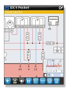
The wiring diagrams can be viewed directly on the instrument monitor. The areas of interest can be enlarged and components selected for greater detail.
