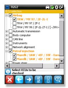
The IDC4 software, thanks to the TGS2 function, can automatically analyse all the recognized vehicle's control units, without having to self-diagnose each system individually.
