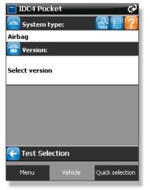
Once the systems family has been defined, choose the system and version with which the specific vehicle is equipped. At this point, you gain direct access to the available self-diagnosis tests.
