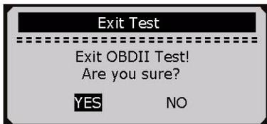
3) If you do want to exit OBDII test, press **ENTER/EXIT** button.
