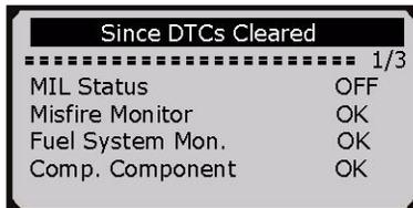
5) If the vehicle supports readiness test of “**This Drive Cycle**”, a screen of the following will be displayed:
