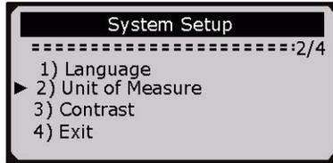
2) From Unit of Measure menu, use SCROLL button to select the desired unit of measurement.
