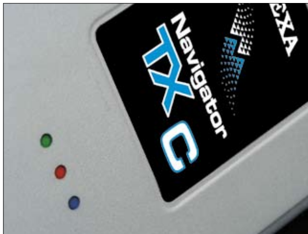
Tool operating status LEDs: green indicates that the tool is on, red indicates communication with the USB port, and blue communication via Bluetooth .
